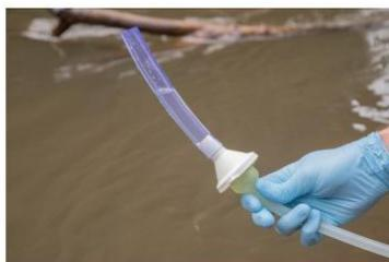
3. When "low flow" alarm sounds or target volume is reached, quickly invert the filter housing and elevate it to filter all remaining water in housing and clear the suction line.
