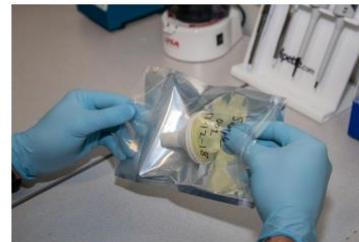
10. Once in the laboratory for DNA extraction, remove the filter housing with the preserved 47mm eDNA membrane from the storage bag.
