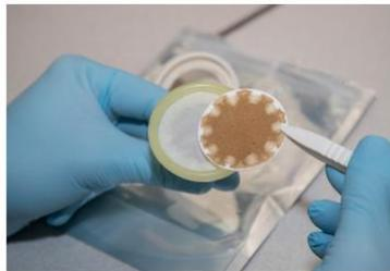
12. The eDNA filter membrane can then be removed from the housing using forceps for DNA extraction. The filter backer will remain stuck to the housing. All elements other than the eDNA filter membrane can then be discarded.
