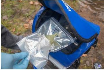
8. Label the sample bag and place sample in a field storage container at ambient temperature.
