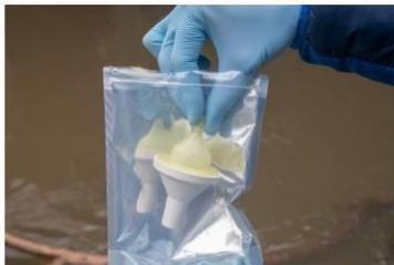
6. Place the self-preserving filter housing back into the original packaging. Minimize excess moisture on the outside of the filter housing. A light shake can remove water droplets.
