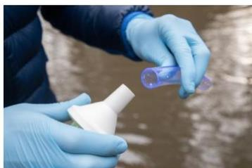
5. Remove the extension tube and discard in an appropriate field waste container.
