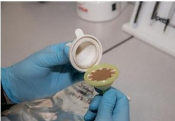
11. Open the filter housing using the pull-tab and reveal the eDNA filter membrane.
