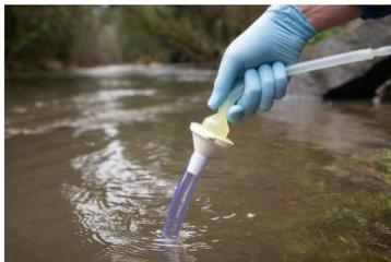
2. Attach suction tubing to the filter housing and activate pump to begin filtration.
