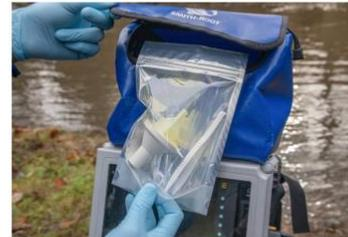
1. Open a sample packet containing a 47mm self-preserving filter housing and attach the extension tube to the housing. Save the foil pouch for subsequent filter storage.
