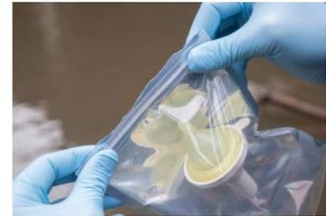
7. Reseal the foil pouch with the zip-type sealing strip. The filter housing material will immediately begin preserving the captured eDNA by desiccation.
