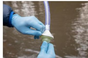
4. **IMPORTANT: Crack the seal (do not open) and allow the pump to run for approximately 20 seconds to air dry the filter membrane. Excess moisture will prevent thorough desiccation and eDNA preservation.**
